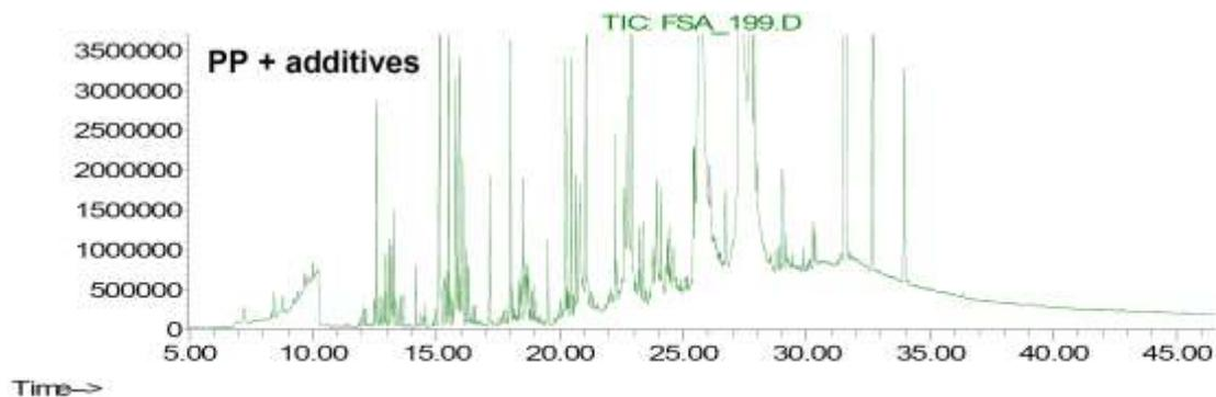
**Figure 2: A plastic organic extract (Polypropylene+additives, extracted with ethanol) analyzed using gas chromatography-mass spectrometry (GC-MS). Each peak represents a different chemical (reproduced from (Bradley and Coulier 2007)).**
